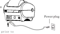
Note: Please switch OFF printer power switch prior to plug in the power cord to printer power jack.
